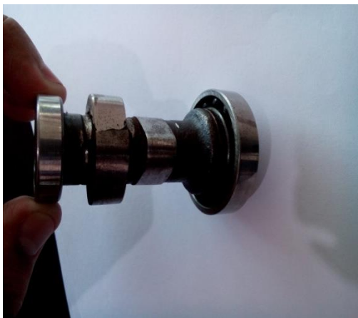
Figure 5: Camshaft of compressed air engine with four lobes
