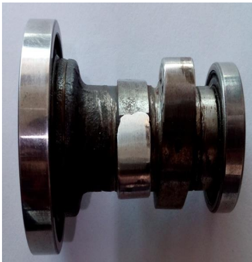
Figure 4: Camshaft of an engine with two lobes
